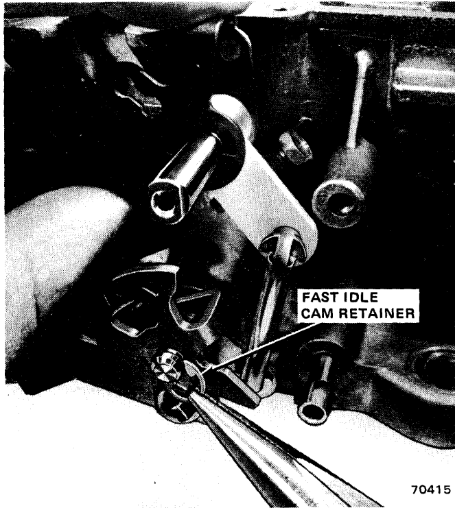
Fig. 4-98 Removing Fast Idle Cam Retainer
